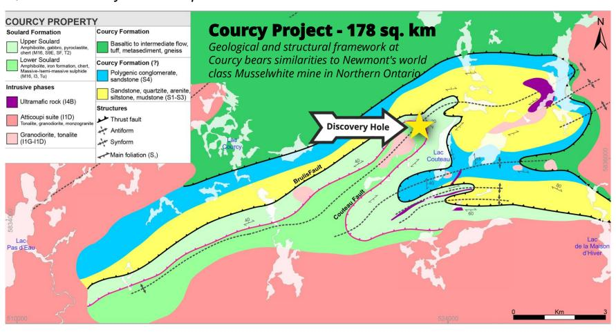
Drilling has targeted gold mineralization now interpreted to be associated with **the Couteau** and Brulis thrust faults that extend for more than 20 km. 2006 discovery hole drilled by SOQUEM was the last of only 8 shallow drill holes ever completed at this under-explored project.
